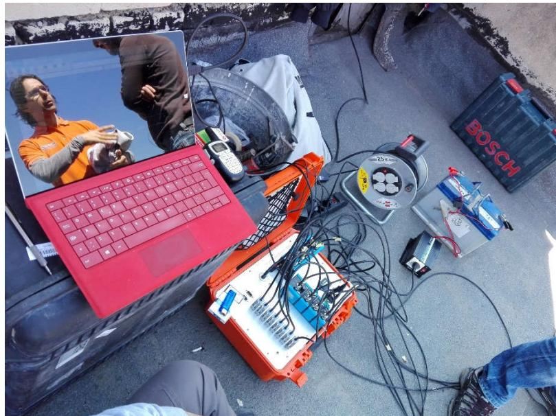
Images 23 and 24. Sensors and data acquisition system
