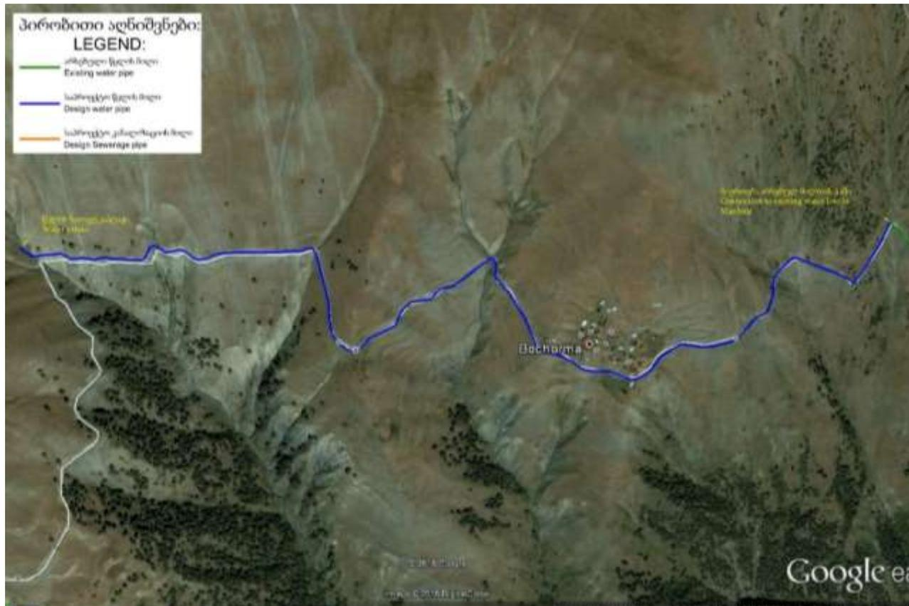
Map 3: Arrangement of water supply system (pipeline, reservoir) and necessary connection infrastructure for existing water pipeline; arrangement of cost and energy efficient sewerage treatment unit (Chlorination plant, septic and sewerage sand filter) for hotel Duruji
