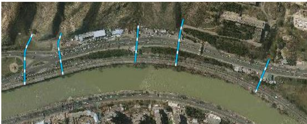
Figure 12: Intersection of the project zone with the storm water pipes
