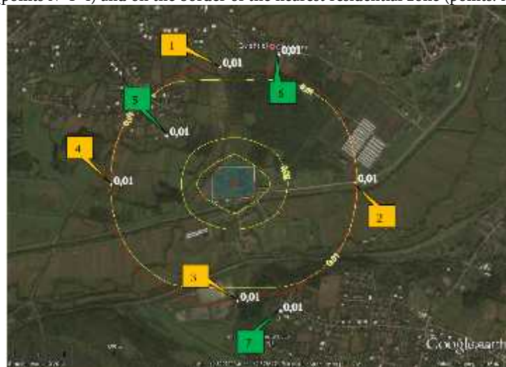
The maximum concentrations of Hydrogen sulphide (code 333) on the border of 500 meters zone (points № 1-4) and on the border of the nearest residential zone (points. № 5-7).
