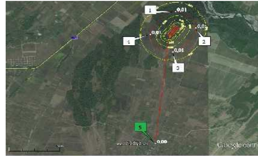
Maximum concentrations of total impact of the 6003 group (codes 303 +333) on the border of 500 meters zone (control points № 1,2,3,4) and on the border of nearest settlement (point № 5)
