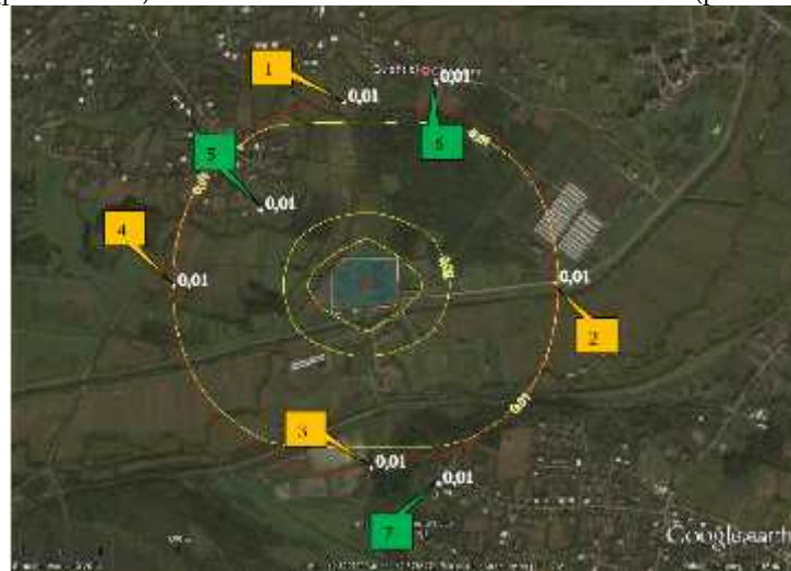
The maximum concentrations of Hydrogen sulphide (code 333) on the border of 500 meters zone (points № 1-4) and on the border of the nearest residential zone (points. № 5-7).
