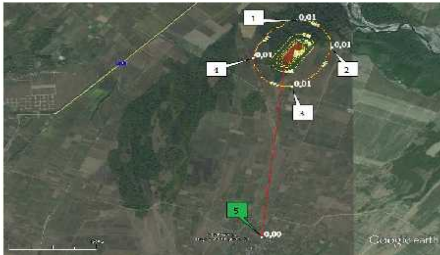
Maximum concentrations of hydrogen sulfide (code 333) on the border of 500 meters zone (control points № 1,2,3,4) and on the border of nearest settlement (point № 5)
