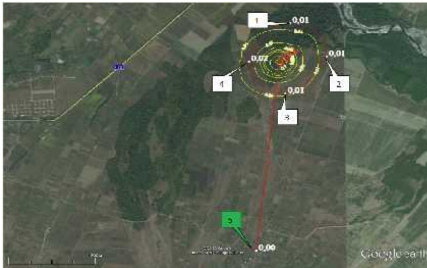
Maximum concentrations of suspended particles (code 2902) on the border of 500 meters zone (control points № 1,2,3,4) and on the border of nearest settlement (point № 5)
