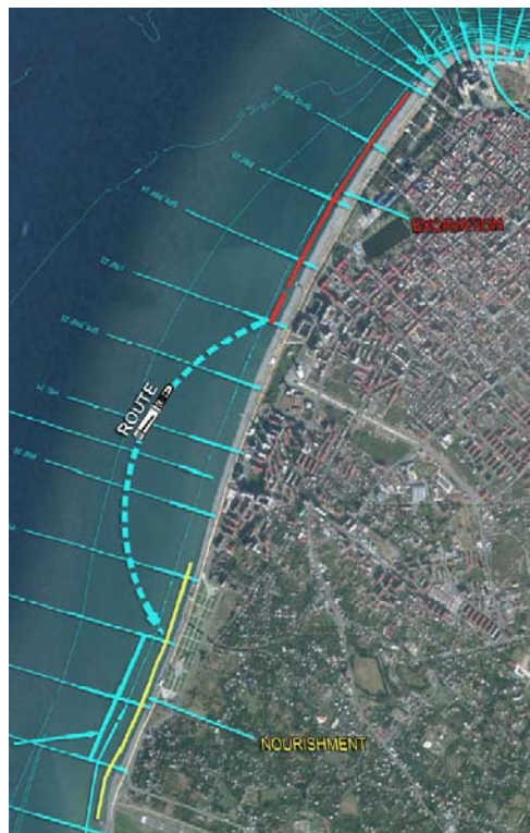
Fig. G-2: Schematization of the excavation – nourishment process
