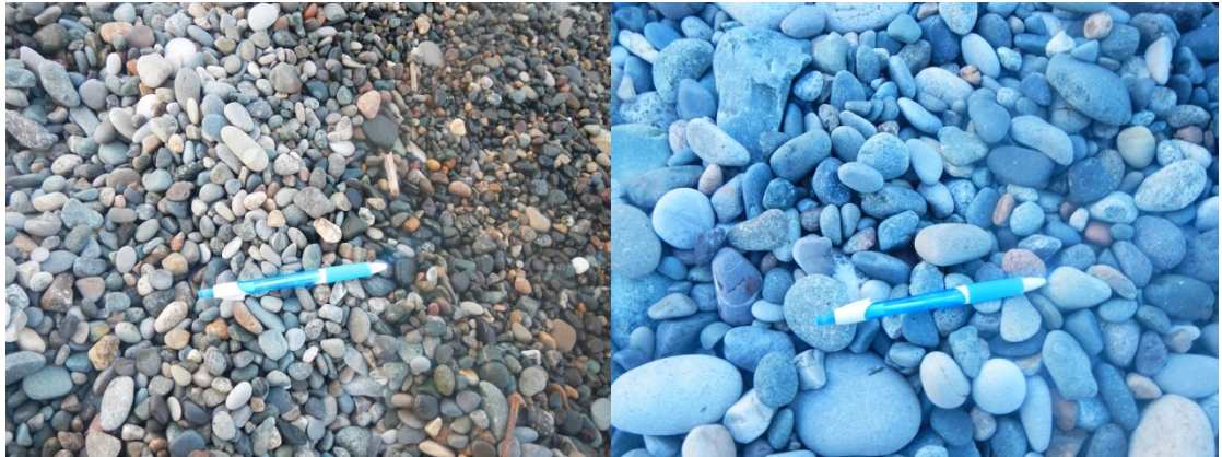
Fig. E-13: Cobbles close to the water line (left) and on the upper part of the beach (right)
