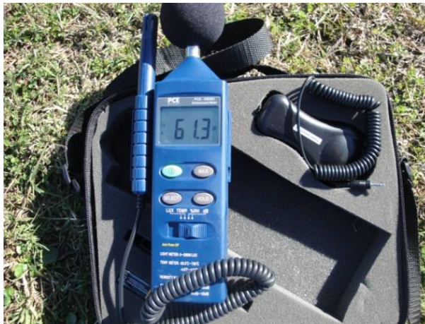
Fig. 4.3. Noise-measuring device PCE-EM882
