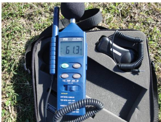
Fig. 4.3. Noise-measuring device PCE-EM882
